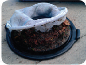
Filtering options 105, 250 or 1000 microns filter bag
