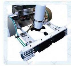
Robot frame is ultra-resistant ultra-light marine quality stainless steel with anti-corrosion warranty
